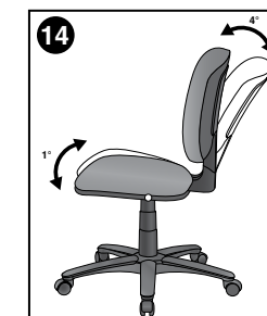
14 Auto Adjusting Synchro Tilt This self adjusting control uses your weight to balance the force needed to recline the back. Back tilt is controlled by a single lever which will lock in 5 positions. When tilting the seat tilts at a 4-to-1 ratio to the back.
