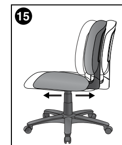
15 Seat Slider Allows adjustment of seat to move forward and back to its original position.
