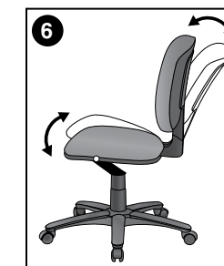
6 Mid-Pivot Knee Tilt Pivot point located slightly ahead of center of gravity (white dot indicates pivot point). Allows user to recline at a slightly more relaxed angle than conventional center tilt.
