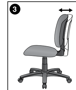
3 Seat Depth Adjustment Positions chair back relative to seat to reduce pressure on the buttocks and thighs for both taller and shorter users.
