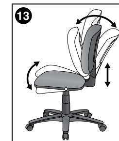
13 Multi-Function Three levers to modify angle of back relative to the seat, control tilt and forward tilt for keyboard intensive activities. Tilt is free float or locking within a fixed range. This control may also have ratchet back height adjustments.
