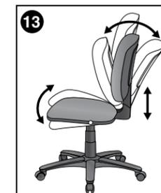
**13 Multi-Function** Three levers to modify angle of back relative to the seat, control tilt and forward tilt for keyboard intensive activities. Tilt is free float or locking within a fixed range. This control may also have ratchet back height adjustments.
